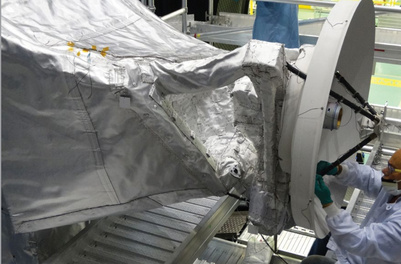
The BepiColombo High Gain Antenna Mechanism Assembly Qualification Model being prepared for thermal testing at ESTEC
