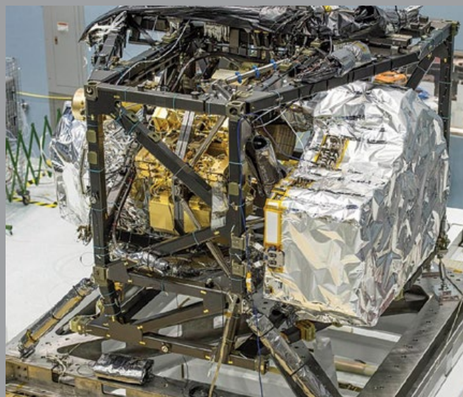
Integrated Science Instrument Module in flight configuration after reinstallation of all the upgraded instruments (NASA/C. Gunn)
