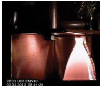
Test-firing of world’s first 3D-printed thruster with platinum combustion chamber and nozzle (ESA/Airbus Defence & Space)
