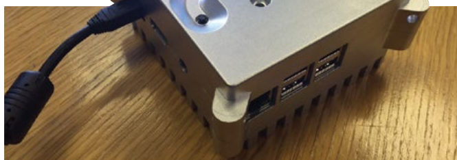
↑ A space-rated version of 'Raspberry Pi' mini computer that Tim will use to run code written by students
